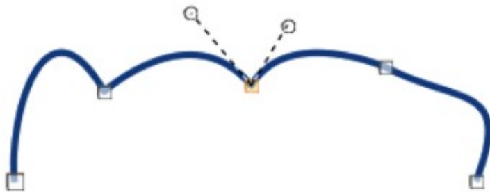
Figure 303: Example corner point
