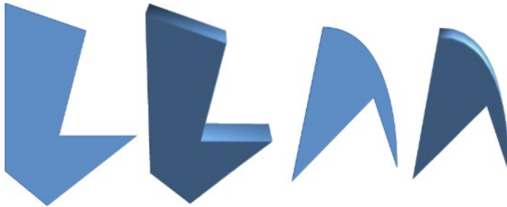
Figure 171: Example of 3D conversion using extrusion
