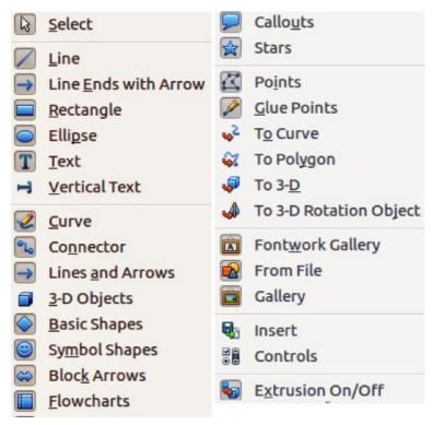
Figure 12: Tools available for Drawing toolbar
