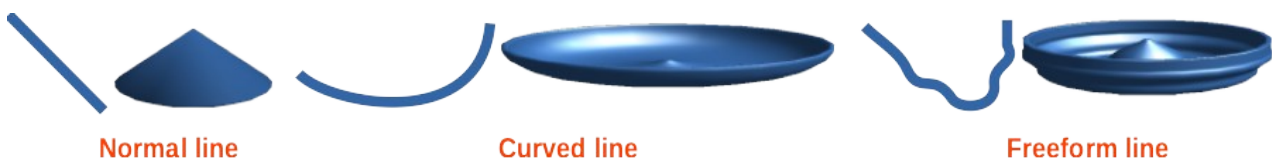
Figure 8: Examples of To 3D Rotation Object conversion
