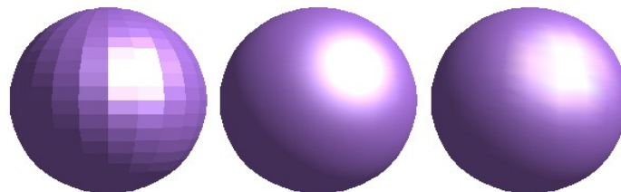
Figure 153: Flat, Phong and Gouraud shading
