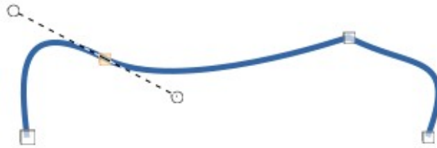
Figure 309: Example of a smooth transition point
