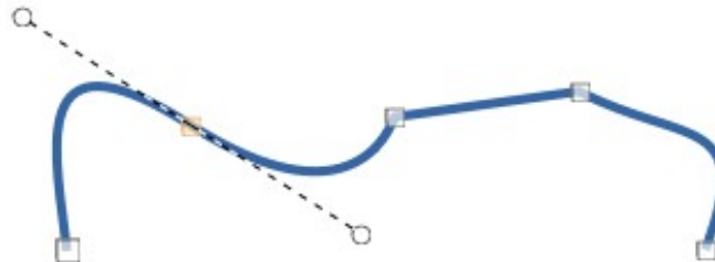
Figure 41: Example of a symmetrical transition point
