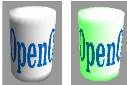
The *Specular color* simulates the reflecting capacity of the surface. The position of the illuminated point is determined by the setting of the first light source.
