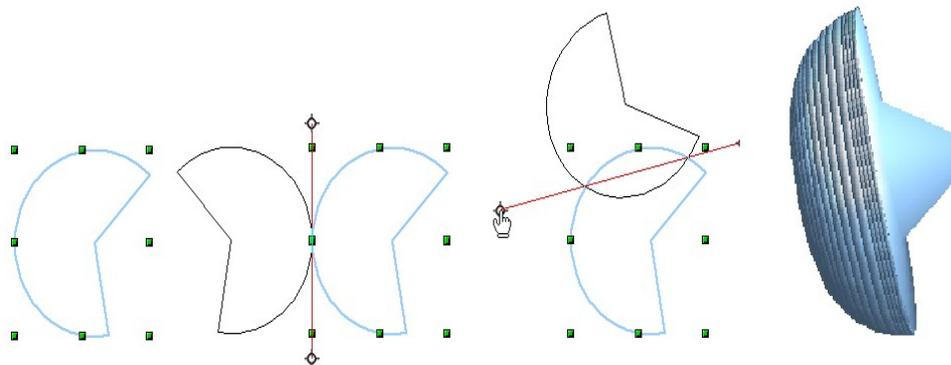
Figure 3: Rotation body created using variation 2.2
