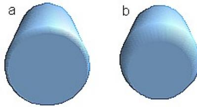
Figure 16: Edge rounding of 10% (a) and 30% (b)
