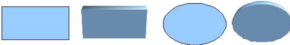
Figure 1: Extruding 3D objects from 2D surfaces
