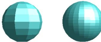
Figure 20: Sphere from 10 segments (left) and 25 segments (right)
