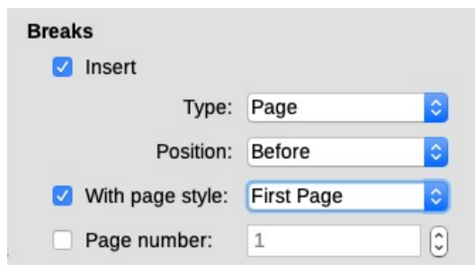
Figure 11: Breaks section of Text Flow tab of Paragraph Style dialog for Heading 1
