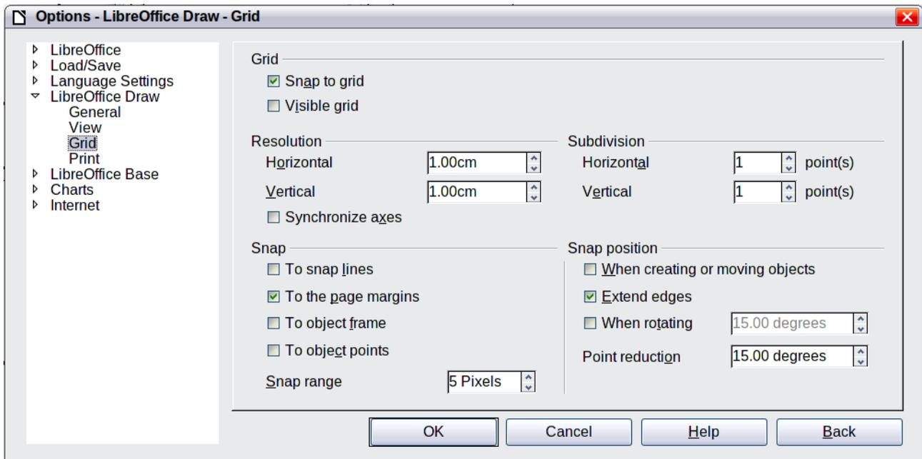
Figure 8: Configuring the grid
