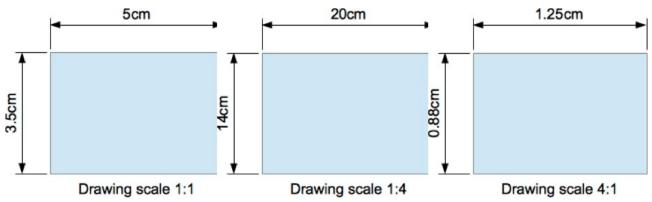
Figure 291: Examples of drawing to scale
