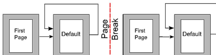
Figure 164: Dividing a document into chapters using page styles
