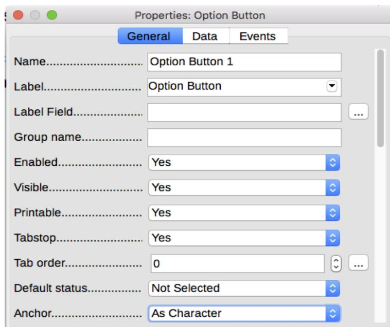
Figure 397: Example of the Properties dialog for a form control
