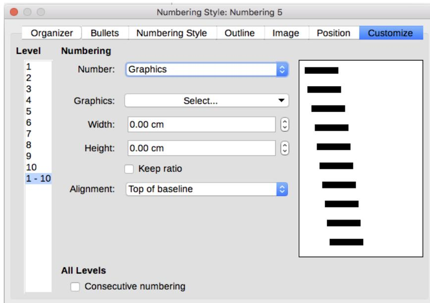
Figure 267: The fields for using a picture as a bullet appear after you have selected *Options > Number > Graphics or Linked Graphics*
