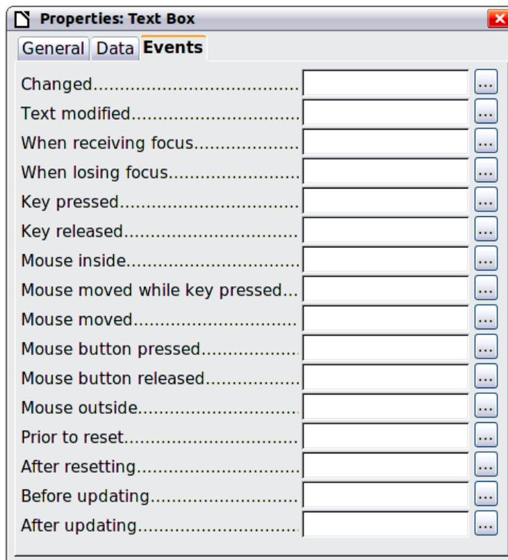
Figure 411: Control properties, Events tab
