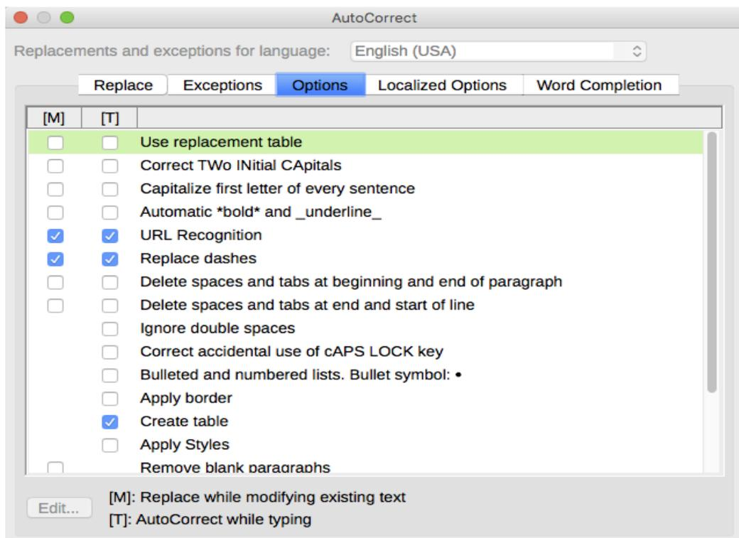
Figure 74: Autoformat choices on the Options page of the AutoCorrect dialog
