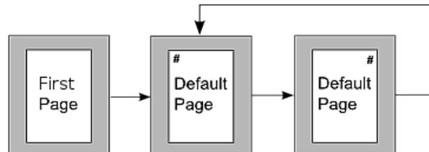
Figure 167: First Page and then the Default page style with different headers for alternate pages
