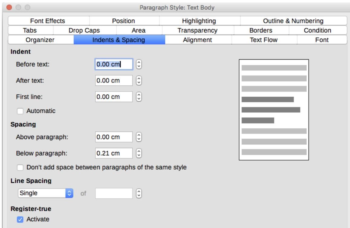
Figure 198: Settings on the Indents and Spacing page of a paragraph style dialog
