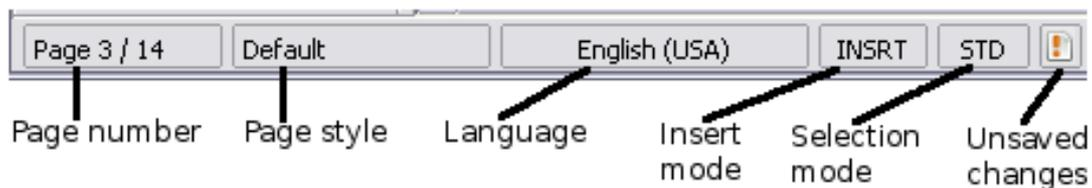
Figure 7: Left end of status bar in Writer
