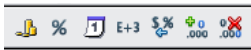
Figure 16: Number format icons. Left to right: currency, percentage, date, exponential, standard, add decimal place, delete decimal place.
