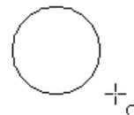
Release the mouse button and move the cursor to the position where you want the arc to start. In the status bar, you can measure the actual angle in degrees. Single-click this point; the circle (or ellipse) disappears and moving the mouse creates the arc. Again, the status bar shows the current angle.
