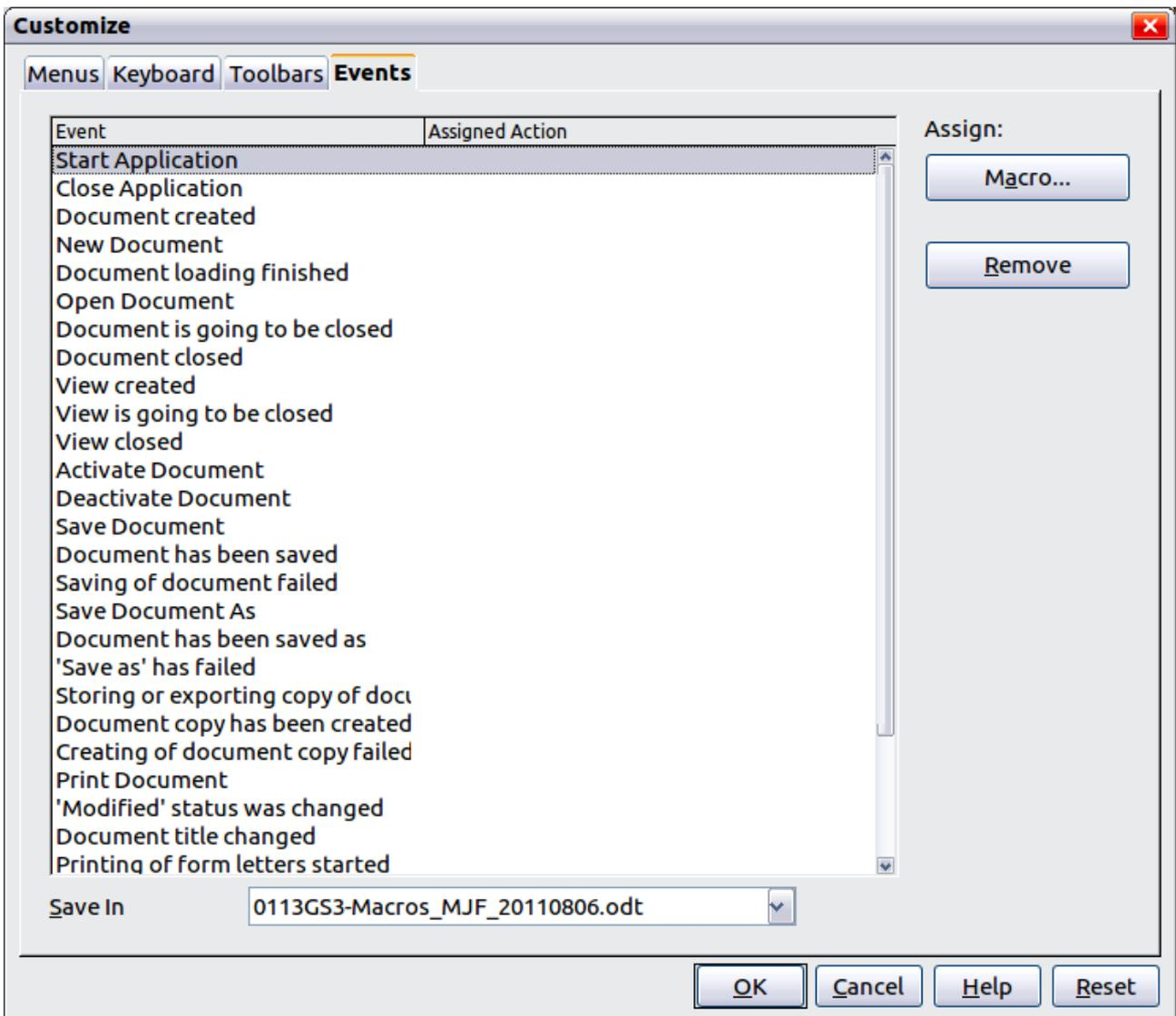
Figure 13: Assign macro to an application level event
